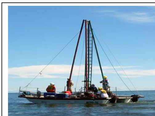
LRC (Limnological Research Center in Minneapolis) coring rig used to recover 10 cores from around the Lake of the Woods last summer
