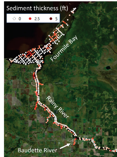
Soft sediment thickness measured by manual soundings
